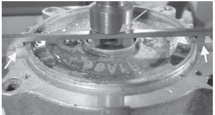
Figure 2 Gage Positioned on Motor (PICTURED WITHOUT PUMP END)
